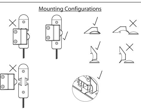
When installing this contact, it is important that you correctly align the contact and the magnet. A roller shutter door with excess side movement must be corrected prior to installation. The two units have location aids to ensure correct line up. When aligning you must check that the supplied magnet triggers the alarm circuit only. If the magnetic detection circuit is wired in, the unit will signal a tamper condition if a roque magnet is introduced.
